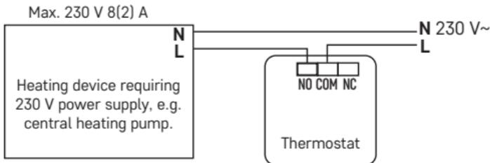
\* When connecting a cooling device to the thermostat, connect the „L“ phase conductor to the „NC“ terminal.
